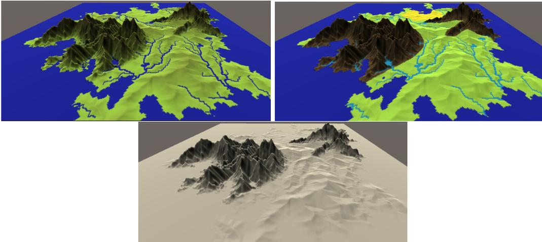
**Figure 4.14** Highlighting different aspects of the algorithm using different texture modes. Top-left: Normal mode (blue for all types of water bodies, gradient for landmass based on height), top-right: Region mode (separate colour for each region: Dark blue for ocean, light blue for rivers and lakes, brown for mountains, yellow for desert, green for flatland), bottom: Height mode (black and white gradient based on the normalized height value).
