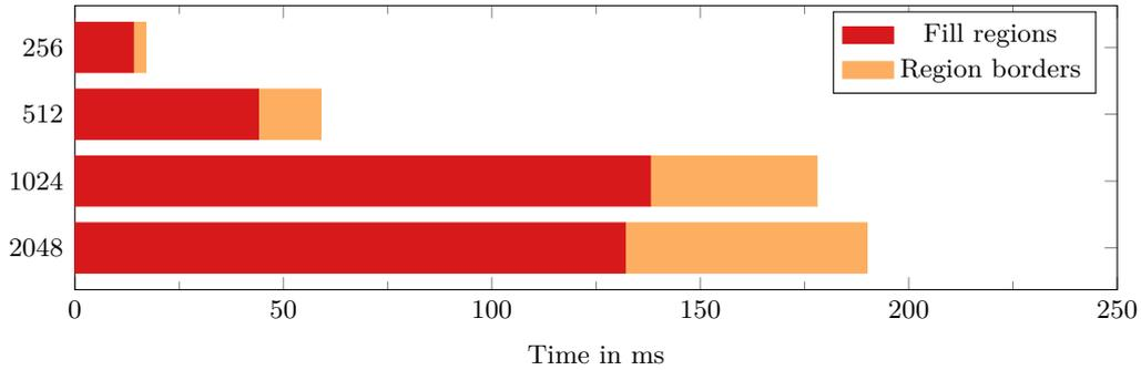
**Figure 5.11** Plotted average times for region filling and calculating of region borders against grid side length  $n_c = 256, 512, 1024, 2048$ . The data is taken from table 5.10. Note that the time does not increase as expected. This is due to less landmass being generated for  $n_c = 2048$  in comparison to lower values of  $n_c$ . This leads to lower calculation time for region separation.
