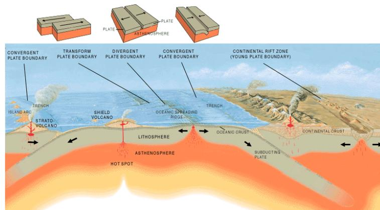
**Figure 2.13** A schematic showing the different types of plate boundary interactions (Vigil, 1997)
