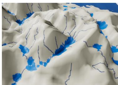
**Figure 3.1** Section of a river network with lakes generated with A\*. Dark blue depicts river cells resulting from the shortest path calculated. The lighter blue areas represent the areas searched by the path finding resulting in lakes.
