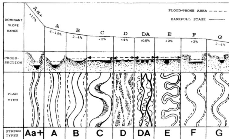
**Figure 2.11** Classification of rivers by cross section and plane view (Rosgen, 1994)
