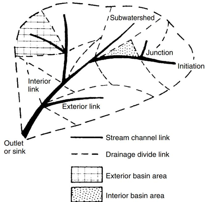
**Figure 2.9** A schematic showing the general structure of a drainage basin (Lin et al., 2006)
