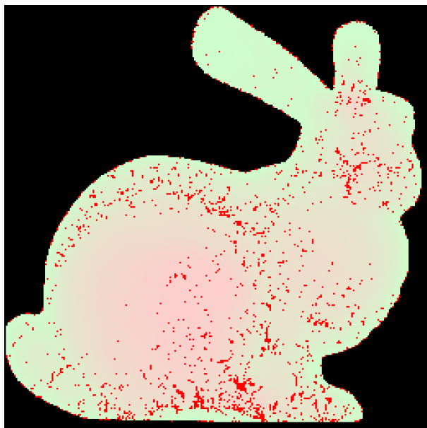
Figure 5.5: Difference between a non-optimized fast packing and a more optimized packing. Red pixels have more than 6% difference.
