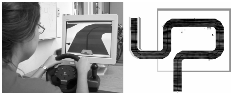
FIGURE 1. (A) Participant driving the wheelchair simulator. (B) Top view of the pathway the participants were required to complete.
