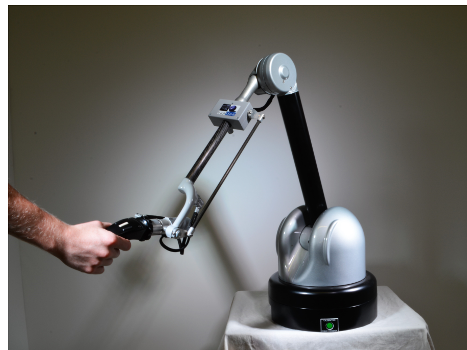
Virtuose (6 DOF's tracking, 3 DOF's force)
