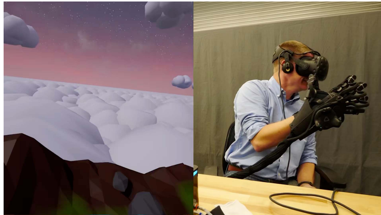
HaptX (armored exoskeleton, 100 actuators)
