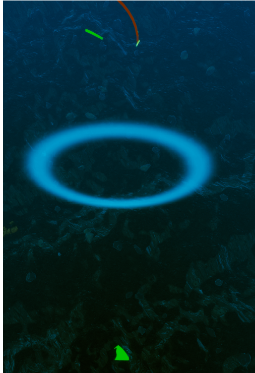
Figure 3.4: The results of the echo sounder, the green dot is the predicted position if the current AUV position is used as the origin position and a downward direction (0,0,-1) , and the depth (in cm) of the echo sounder (The green dot is only used for debugging and is not displayed in the simulation). The white circle is the ripple effect that we use to visualize the "EchoBeam" (see chapter 6.4.2 for more information), and the green and red lines are the path visualization (see chapter 3-Trajectory for more information).
