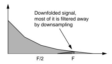
FIGURE 197. Super-sampling significantly reduces aliasing
