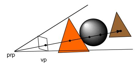
FIGURE 199. Ray-casting in a scene. A ray is formed through prp and a pixel in the image plane.
