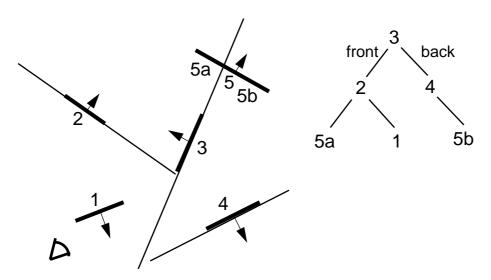
FIGURE 125. BSP tree example (Adapted from Foley, van Dam [27].)
