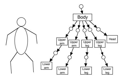
FIGURE 145. Hierarchical representation of a human body
