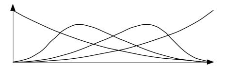
FIGURE 65. Blending functions for a 4-point Bézier curve
