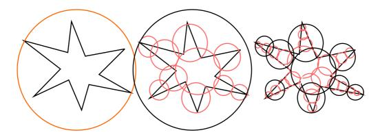
FIGURE 159. An example of a hierarchical collision detection system
