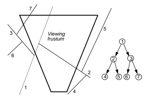
FIGURE 130. Clipping using a BSP tree
