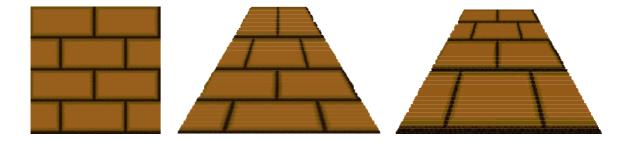
FIGURE 190. A texture, mapped on a polygon with affine and perspective correct mapping, respectively
