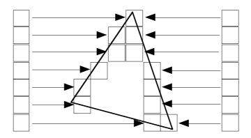
FIGURE 186. Filling the span buffer
