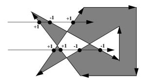
FIGURE 178. The zero winding number test: Count intersections as +1 or -1
