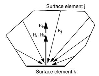
FIGURE 208. The light energy emitted from k is given by its own emission  $\boldsymbol{E}_k$  and incoming light energy  $\boldsymbol{H}_k$
