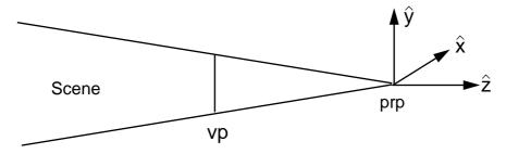
FIGURE 32. The camera model, with optical center prp and viewing plane vp
