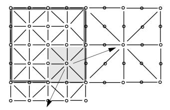
FIGURE 142. When the shaded square is drawn, the algorithm must test the two closest neighbors of its parent square (gray frame)
