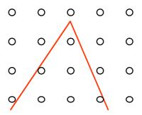
FIGURE 176. Pixels are mapped to points according to the pixel definition, which gives clear decisions
