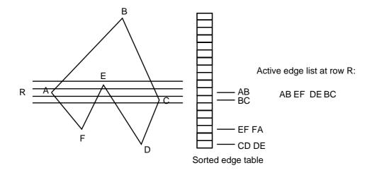
FIGURE 180. Scan-line polygon fill
