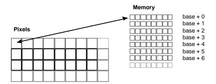
FIGURE 4. With chunky pixels, each pixel is one single chunk of memory
