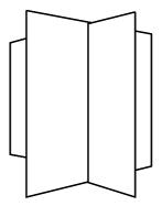
FIGURE 139. A multi-face billboard, with polygons in two or three different planes, does not need any rotation.
