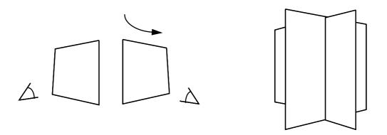
FIGURE 135. A billboard (left) is a single polygon always facing the viewer. Two or three polygons, with no rotation to face the viewer (right) gives higher realism
