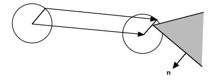
FIGURE 162. A case where the speed vector doesn't intersect any polygon, but we should still detect a collision!
