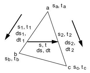
FIGURE 189. Affine texture mapping, linear interpolation
