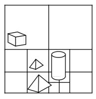
FIGURE 203. Subdivision of space into a quadtree to simplify searches
