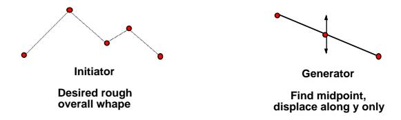
FIGURE 85. Hinted random midpoint displacement method
