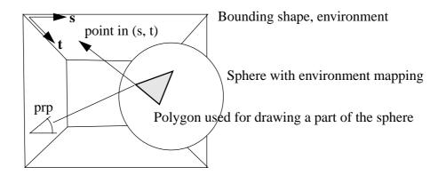
FIGURE 111. Environment mapping
