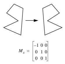
FIGURE 24. Mirroring along the X axis
