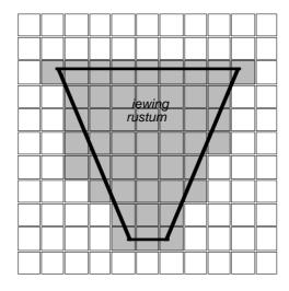
FIGURE 127. Frustum culling in a grid is particularly simple.
