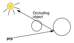
FIGURE 202. The shadow ray tests whether or not a surface point is visible from the light source or not
