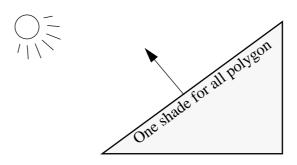
FIGURE 42. Flat shading, calculate one shade for entire polygon
