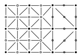
FIGURE 141. A possible way to patch the edge between areas of different resolution
