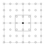
FIGURE 74. Four Bézier patches connected. The nine center control points must be in a plane
