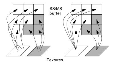
FIGURE 198. Comparison supersampling vs multisampling
