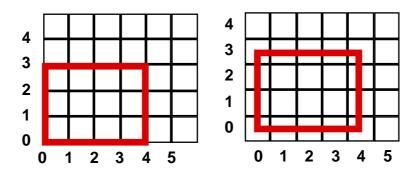
FIGURE 173. The polygon's position varies with the pixel definition
