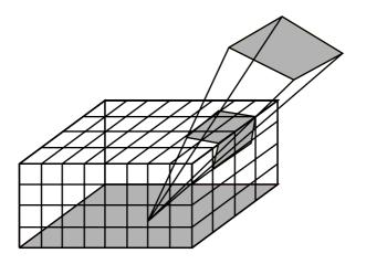
FIGURE 209. Enclosing half cube for approximation of form factors
