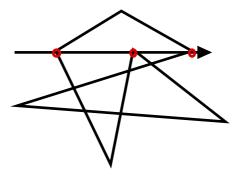
FIGURE 181. How do you count edges for a scan-line that passes through vertices?
