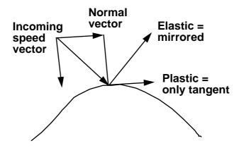
FIGURE 164. Simple particle-surface collision handling
