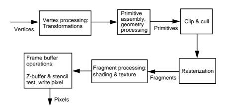
FIGURE 34. The OpenGL pipeline (simplified)
