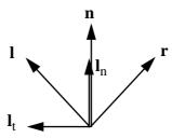
FIGURE 11. Reflection of a vector by projection on the normal vector
