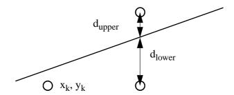
FIGURE 169.  $d_{upper}$  and  $d_{lower}$  are the distances from the candidate pixels to the line
