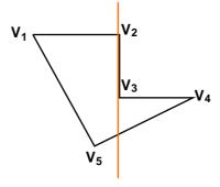
FIGURE 15. The vector methods uses a polygon branch near a concave vertex as splitting vector
