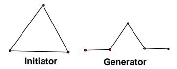
FIGURE 79. A self-similar geometric fractal is defined by an initiator and a generator
