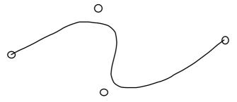
FIGURE 64. The 4 points are blended together using 4 blending functions
