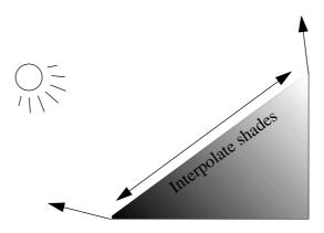
FIGURE 46. Gouraud shading, calculate light at vertices, interpolate shades
