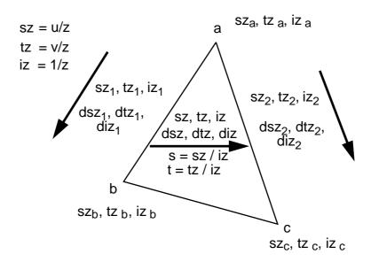
FIGURE 191. Implementation of perspective correct texture mapping
