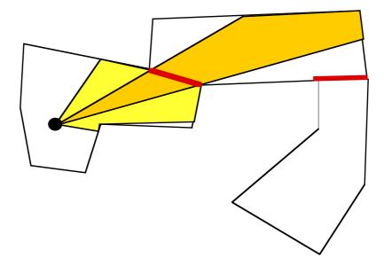
FIGURE 131. Example of Portals. The thick "walls" are portals, openings into the next room.
