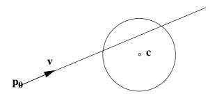
FIGURE 10. Intersection between a line (ray) and a sphere
