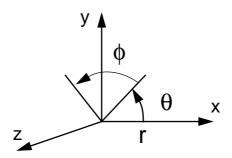
FIGURE 61. Polar coordinates: positions are given as a radius placed on the X axis, rotated around Z by  $\theta,$  and then rotated around X by  $\phi.$
