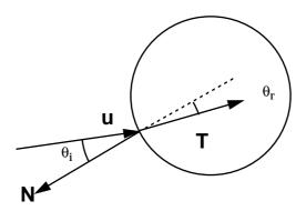
FIGURE 201. Refraction
