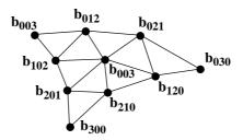
FIGURE 75. Control points used by a curved PN triangle
