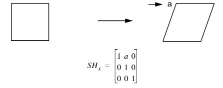
FIGURE 25. Shearing along the X axis
