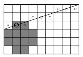
FIGURE 171. Drawing wide curves using a pen shape
