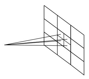
FIGURE 204. Super-sampling, e.g. 4 rays in a regular pattern
