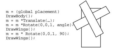
FIGURE 143. Lab-style windmill, code and simplified result
