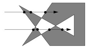
FIGURE 177. The odd-even test: Count the number of intersections
