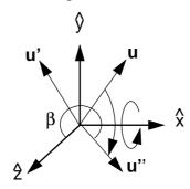
FIGURE 28. The vector u is rotated down onto the XY plane.
