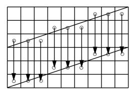
FIGURE 172. Drawing wide curves using two parallel curves
