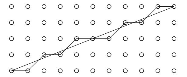
FIGURE 170. Example of line drawing with Bresenham's algorithm
