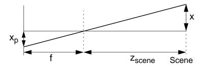
FIGURE 31. Projection geometry of a physical camera
