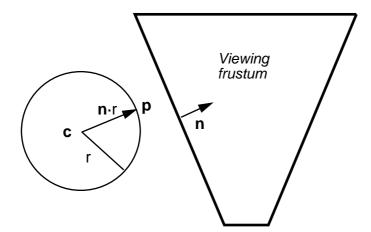
FIGURE 128. Sphere-frustum test used for bounding spheres of objects
