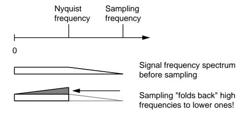
FIGURE 193. Higher frequencies are "folded" over the Nyquist frequency
