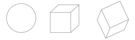
FIGURE 156. The three basic shapes for collision detection: sphere, AABB and OBB
