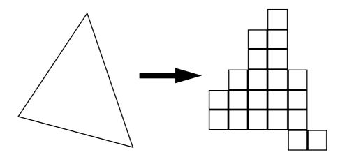
FIGURE 183. Scan conversion: From polygon to fragment (pixel) coordinates
