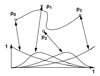
FIGURE 66. The four control points are blended to the spline by the blending functions
