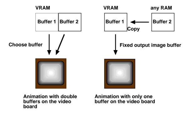
FIGURE 148. Two different cases of double buffering
