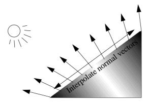
FIGURE 48. Phong shading; interpolate normals, calculate light by pixel
