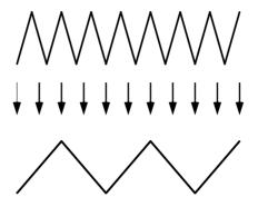
FIGURE 192. Example of how sampling can result in a lower frequency
