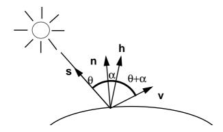
FIGURE 41. Specular reflection calculation using the halfway vector
