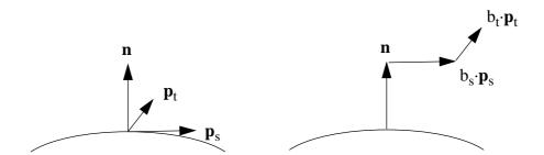
FIGURE 110. Bump mapping. The normal vector is modified by components in u and v direction
