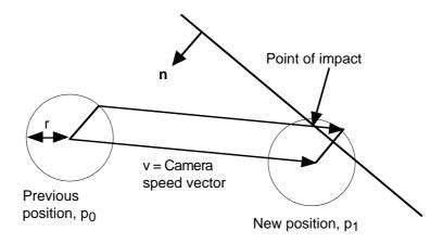
FIGURE 161. Collision camera to (infinite) plane
