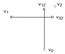
FIGURE 187. dx and dy can be calculated by interpolating the intermediary points v02 and v12 and their intensity values.
