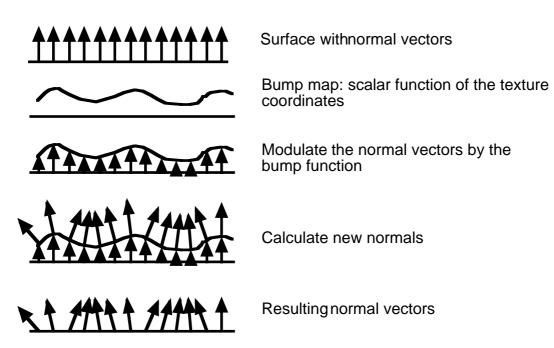
FIGURE 109. Principle for bump mapping
