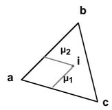
FIGURE 9. Checking if ithe pointy is inside the triangle abc.
