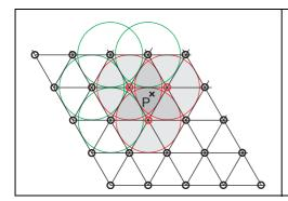
A point P inside a simplex gets contributions to its value only from the three kernels centered on the surrounding corners (shaded, red circles). Kernels at corners farther away (green circles) decay to zero before they cross the boundary to the simplex containing P. Thus, the noise value at each point can always be calculated as a sum of three terms.
