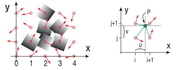
The value of each gradient ramp is computed by means of a scalar product (dot product) between the gradient vectors of each grid point and the vectors from the grid points (i, j), (i + 1, j), (i, j + 1), (i + 1, j + 1) to the point P being evaluated. In equations:
