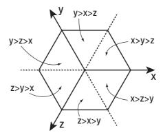
For the 4D case, things become incomprehensible visually, but the methods presented for 2D and 3D generalize nicely to higher dimensions. Sorting the (x,y,z,w) coordinates within the hypercube reveals 4! = 24 possible outcomes for the ordering of the magnitude of the coordinates, and each particular ordering is unique to one of the 24 simplices.
