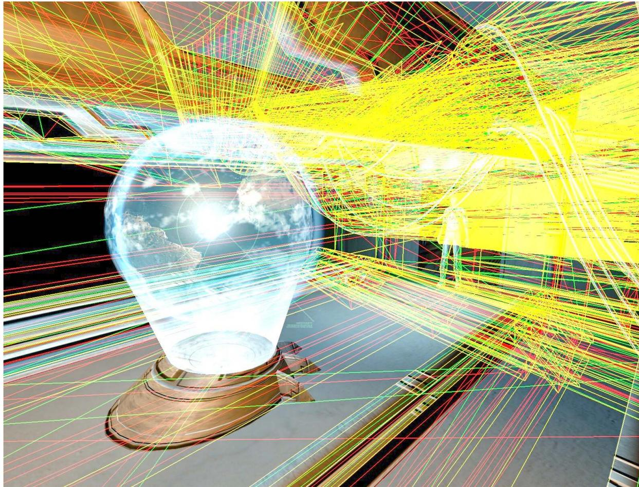
Wireframe shows geometric *complexity of shadow volume* geometry
