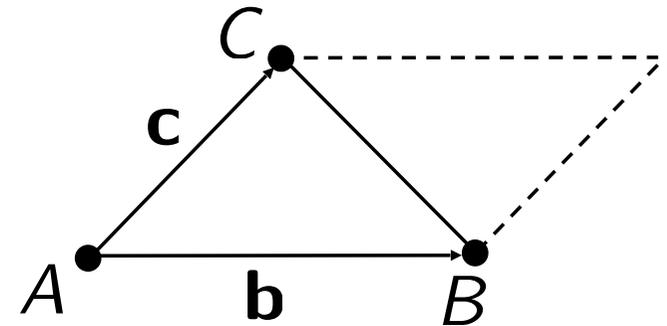
$$= \frac{1}{2} \begin{vmatrix} B_x - A_x & C_x - A_x \\ B_y - A_y & C_y - A_y \end{vmatrix} = \frac{1}{2} \begin{vmatrix} A_x & B_x & C_x \\ A_y & B_y & C_y \\ 1 & 1 & 1 \end{vmatrix}$$
