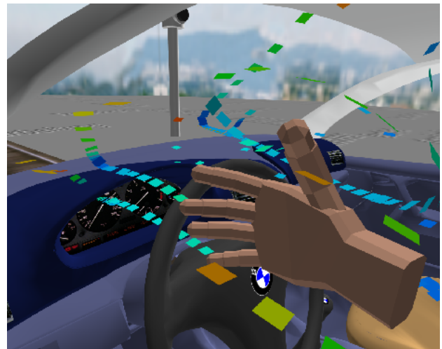
Figure 14: The flow of air particles at the front window, with some fixed particle sources and the hand as a freely movable source. Data courtesy of BMW AG.
