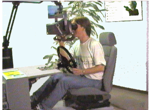
Figure 3: The physical equipment of the BMW virtual seating-buck.
