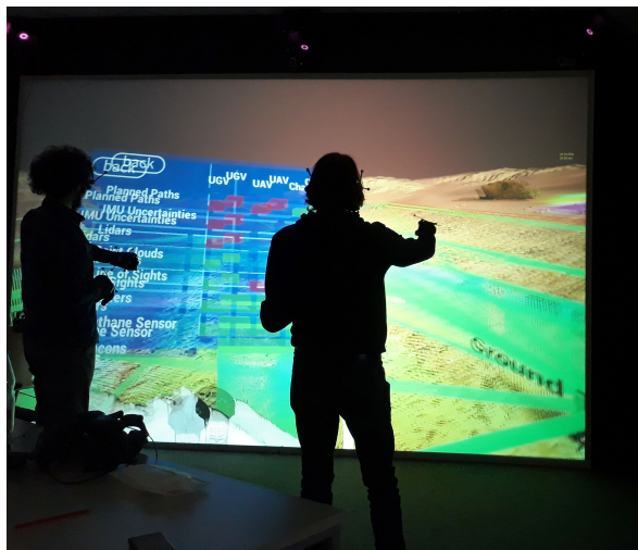
Figure 13: Two users collaborating in front of our multi-user powerwall. The tracking is realized via an Optitrack system.
