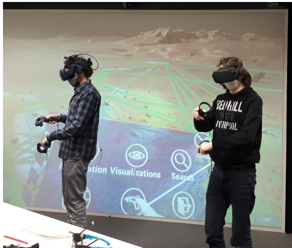
Figure 12: Interaction of two users in the simulated martian environment with HTC Vive HMDs. The view of the right user is also displayed on the screen behind the users.
