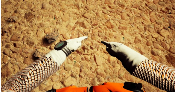
Figure 9: A VR menu can be opened by simply touching the wristwatch of the left virtual hand.
