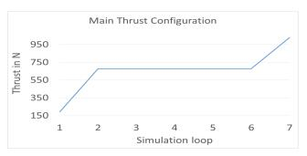
Figure 11: Our approach gradually increases the thrust level until the velocity can be adequately regulated for landing.
