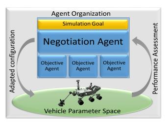
Figure 4: One agent organization is generated for each simulation goals. Each organization searches through the corresponding vehicle parameter space by measuring the vehicle performance and by adapting the configuration until the organization finds a satisfying solution.
