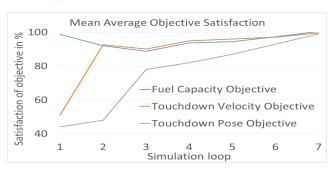
Figure 10: Our approach successfully changes the vehicle configuration in order to increase the simulation goal satisfaction.
