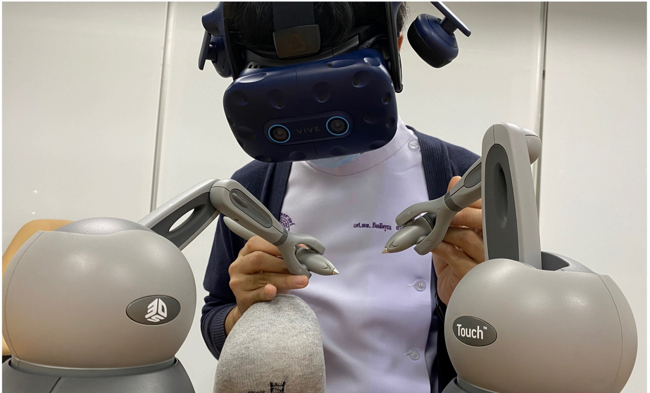
Fig 1. The VR dental surgery simulator is used by a dentistry student to practice root canal access opening on tooth #36. The VR HMD and haptic input/output devices allow for an intuitive control with realistic haptic feedback (in alignment condition). The monitor shows the image that the student is seeing on the HMD.
