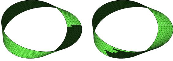
**Figure 2. Some models cannot be oriented consistently. The Möbius strip is a simple example. Here, there are different possible solutions.**
