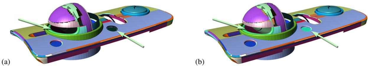
Figure 9. A model with 137 patches: (a) after applying our algorithm with only visibility taken into account; some incorrectly oriented patches are marked with arrows; (b) taking both boundary coherence and visibility into account.
