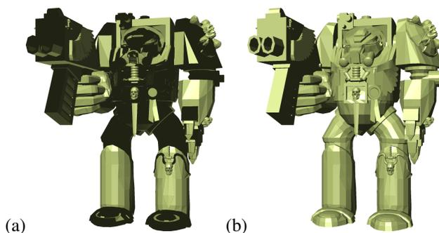
**Figure 1. (a) A model consisting of 2398 separate surface patches with inconsistent orientation; due to the lighting, the faces oriented “backwards” are rendered dark. (b) Same model after applying our algorithm (with exactly the same lighting).**
