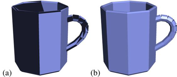
**Figure 6. The coffee mug model used in [9]: (a) polygons are oriented randomly (back-facing polygons are drawn in black); (b) after applying our algorithm all polygons are oriented correctly**
