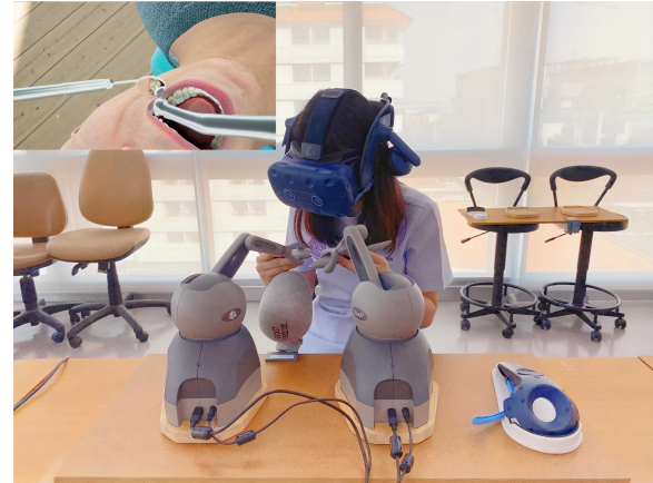
Figure 1: VR Simulator. A student is using our bi-manual VR dental simulator with two force-feedback devices.
