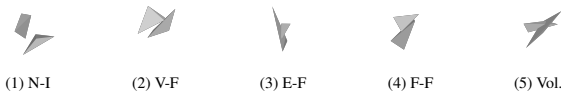
Figure 2: Data Generation Strategies: visualizations of randomly generated .obj tetrahedron-tetrahedron pairs corresponding to five topological configurations. (1) non-intersecting pairs (N-I), (2, 3, and 4) show contact configurations (V-F, E-F, F-F) sampled via constraints, and (5) volumetric interpenetration (Vol.).
