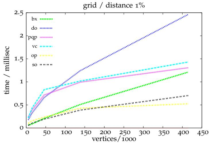
Figure 6.26: The results of the benchmark for the grid scene for a distance of 1% relative to the object size. The  $x$ -axis denotes the number of vertices divided by 1000. In contrast to the lustre scene (Figure 6.25) the running-time seems to increase in  $O(n \log n)$  for all algorithms.
