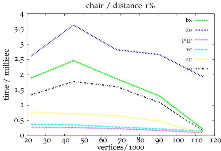
Figure 6.28: The dependency of the collision detection time from the complexity of the models in the chair scene. Again, the distance is fixed to 1% of the object size. In contrast to the castle scene (see Figure 6.27), the collision detection time decreases with an increasing complexity.
