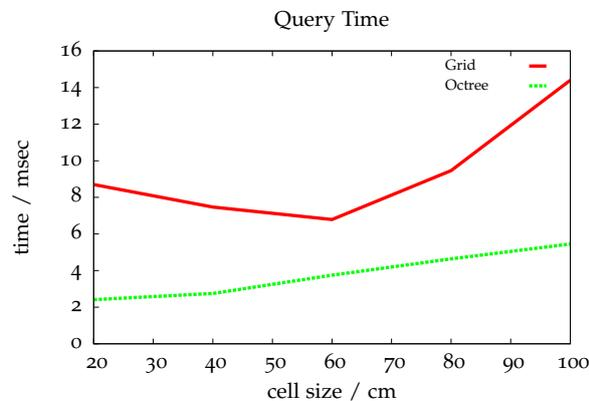
Figure 7.12: Average query time, this means NNS, range query, and exact IST distance computation, for a single point cloud with 270K points. The x-axis denotes different cell sizes of the quadtree and the grid.
