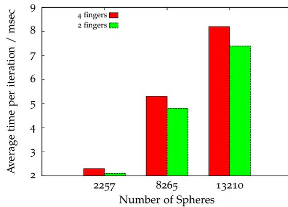
Figure 7.6: Average running-time during for two different movements of the virtual hand. In the first case (red) four fingers of the hand were moved simultaneously, while in the second case (green) only two fingers were moved.
