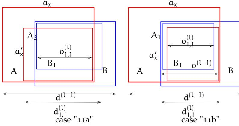
Figure 6.3: Denotations for computing  $d_{11}^{(l)}$  for a child pair. If  $a'_x > o^{(l-1)}$ , the new distance  $d_{11}^{(l)}$  is  $d_{i,j}^{(l-1)} - 2\omega^{(l)}$  with  $\omega^{(l)} = \alpha_x^{(0)} \alpha_x^0 (1 - \alpha_x) = \alpha_x^{(0)} (1 - \alpha_x)$ . In the other case,  $d_{11}^{(l)}$  equals the overlap  $o^{(l-1)}$ .
