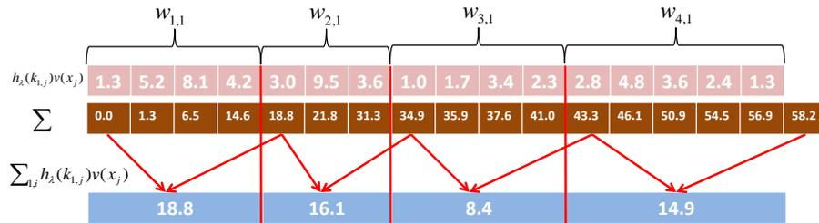
Figure 5.5: In order to compute the new position of the prototypes for the next iteration, we have to determine  $\sum h_\lambda(k_{ij})v(x_j)x_j$ . Therefore, we compute the prefix sum (brown array) for each of the four prototype arrays from Figure 5.4. The differences between the values at the borders directly deliver us the individual sum for each prototype.
