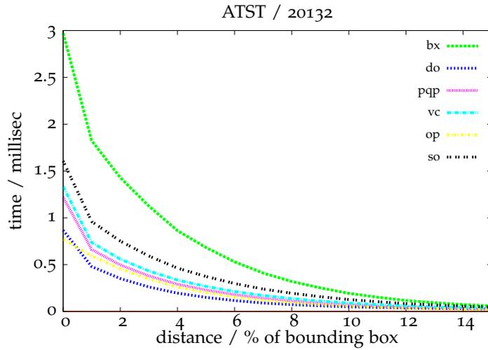
Figure 6.24: The results of the benchmark for the ATST walker with 20132 vertices. Like in the Apollo case (Figure 6.23), the OBB-based algorithms are much faster than the AABB-based libraries.
