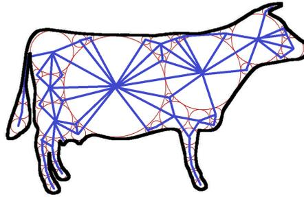
Figure 4.14: Our Protosphere algorithm does not only compute a sphere packing, but also maintains automatically the adjacency between the spheres, the so called *Sphere Graph*.
