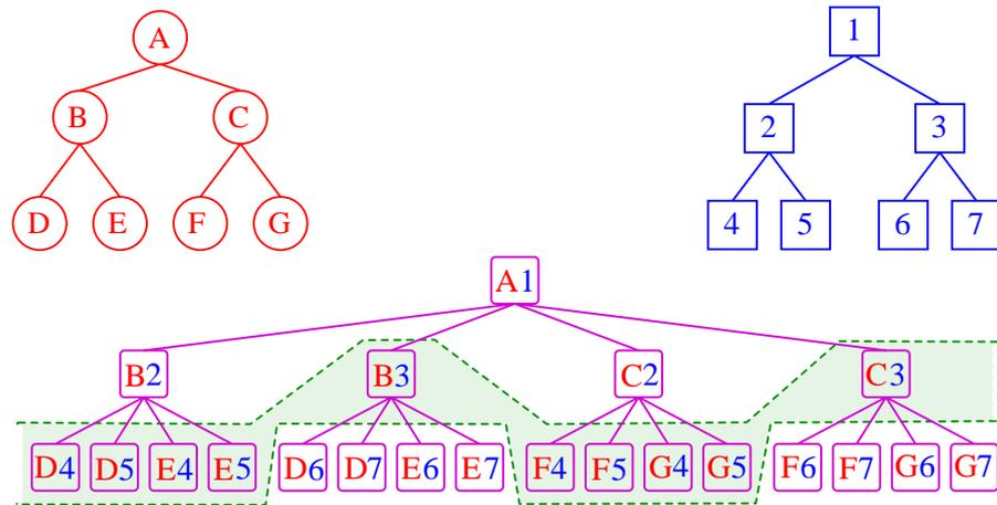
Figure 3.15: The simultaneous traversal of two BVHs results in a BVTT (see Figure 2.4). Those BV pairs, where the traversal stops, build a list in this tree (green). We call it the *separation list*. This list consists of inner nodes, whose BVs do not overlap (B, 3) and leaf nodes, where the BVs are leaves in the BVH that do either overlap or not.
