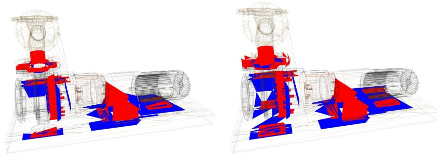
Figure 6.45: The intersecting triangles that were found by PQP (left) and CollDet (right) in a typical CAD simulation. You can see, that CollDet finds much more intersecting triangles.
