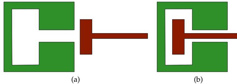
Figure 6.16: The sphere method will find only configuration (a) for the red and the green objects, but it will miss configuration (b).
