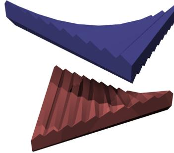
Figure 1.1: The intersection of two Chazelle polyhedra is a worst case for collision detection algorithms.
