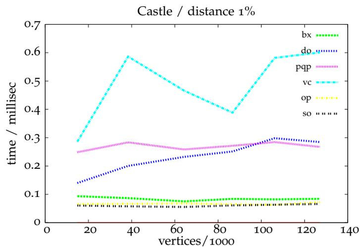
Figure 6.27: The dependency of the collision detection time from the complexity of the models in the castle scene. The distance is fixed to 1% of the object size. The collision detection time seems to be independent of the complexity.
