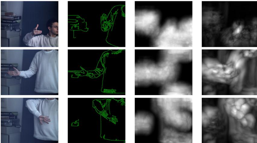
Figure 4.41: Test data set 2 is an open hand rotating in the image plane. Canny thresholds are 20 and 100.
