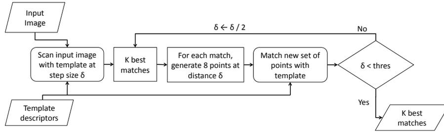
Figure 5.13: The workflow illustrates the massive parallel approach to match a template to an input image using the multigrid approach. Initially, the template is matched to the image at a coarse grid and then successively refined at the most promising candidates.
