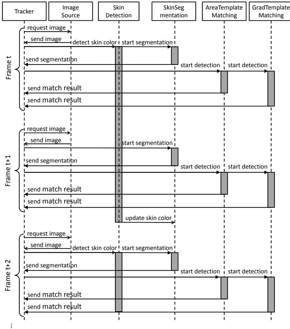
Figure 6.4: Sequence diagram illustrating the most important data flow of our overall hand tracking approach.
