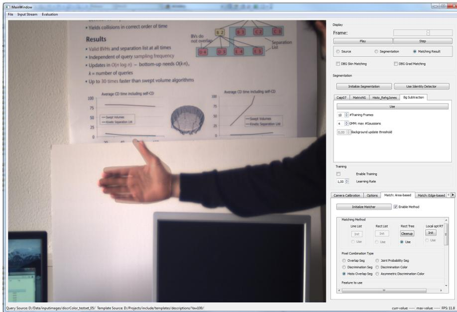
Figure 6.1: Our hand tracking framework. A template set consisting of the open hand with in plane rotation is currently matched to an input image. For the best matching position, an artificial hand model is rendered and superimposed to the original image.
