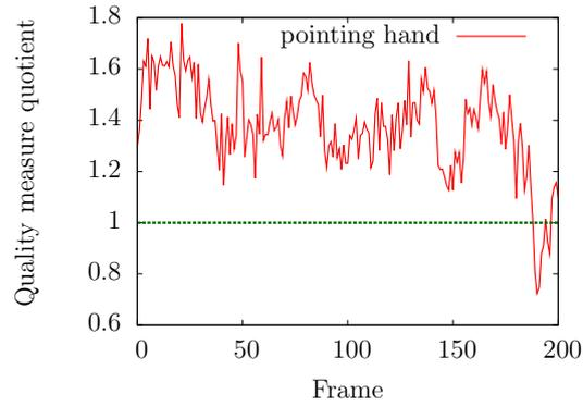
Figure 4.43: The quotient of the quality between our approach and the chamfer based approach is shown. A value greater than 1 indicates that our approach is better.
