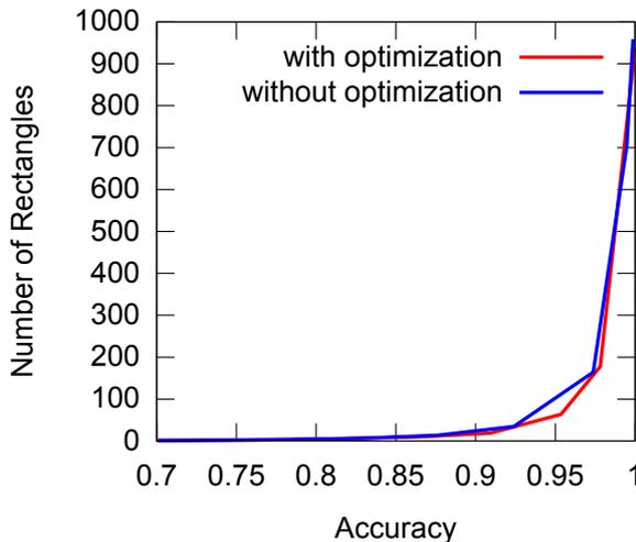
Figure 5.5: Evaluation of the optimized hierarchy: we use a dataset of 100 templates (open hand, in plane rotation) to evaluate our hierarchy optimization that is able to further reduce the number of covering rectangles. The fewer rectangles we have, the less memory the hierarchy consumes and also the faster the matching is.
