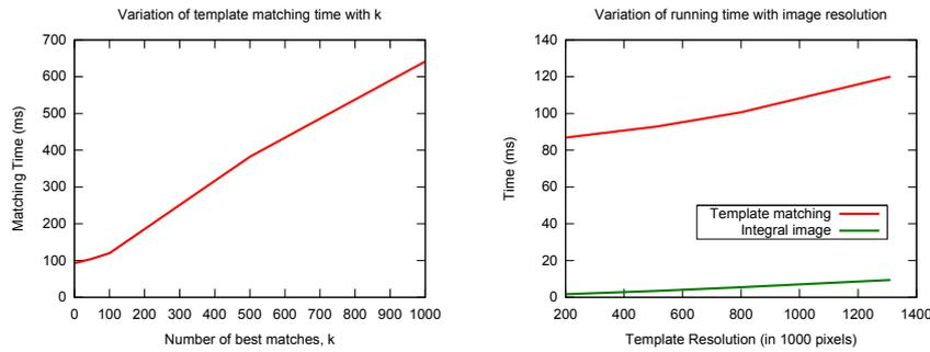
Figure 5.14: The computation time linearly depends on the number of candidates used in the multi-hypothesis tracking as shown in the left image. The computation time also depends linearly on the image resolution (right image).
