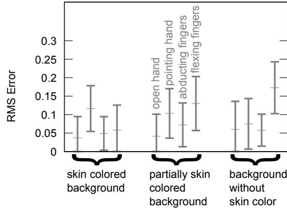
Figure 5.11: Each group shows the results for a specific input dataset. Each bar within each group shows the mean and standard deviation of the RMS error between the brute-force and our coarse-to-fine detection. An RMS error of 1 indicates the maximally possible error.
