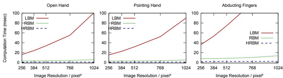
Figure 5.9: Each plot shows the average computation time for all three approaches: LBM [STTC06], RBM (our approach), HRBM (our approach incl. hierarchy). Clearly, our approaches are significantly faster and, even more important, resolution independent.
