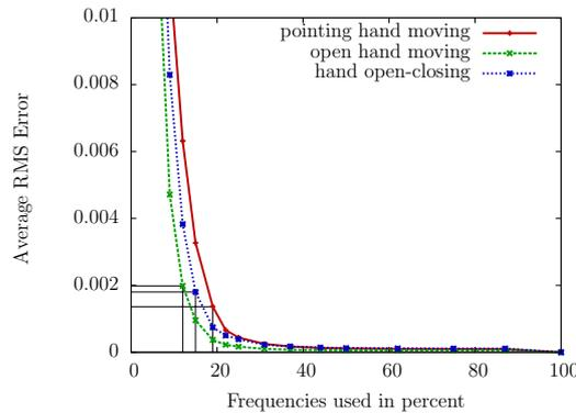
Figure 4.37: For each template dataset: the average root mean square error of combined confidence maps built using templates with only the lower  $f$  percent of the image frequencies. The error is measured relative to the combined confidence map using the uncompressed templates (all frequencies).
