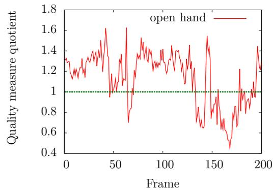
Figure 4.44: The quotient of the quality between our approach and the chamfer based approach is shown. A value greater than 1 indicates that our approach is better.
