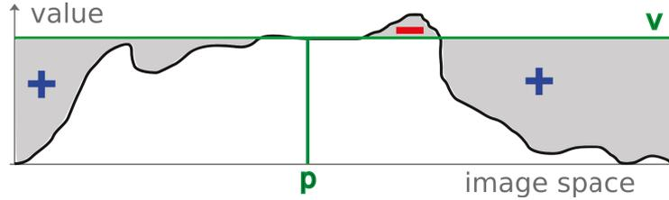
Figure 4.38: 1D example of our quality measure: the true location  $p$  of the target object is determined manually,  $v$  is the value at  $p$  in the combined confidence map. Our quality measure is basically the sum of the signed gray areas over the whole confidence map.
