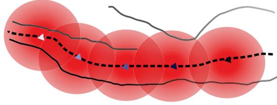
Figure 4.35: We estimate the similarity between a template edge (dashed line) and a query image edge, which is represented by intensities (gray solid curves), by multiplying a kernel that is centered around each template edge pixel (circles) with the edge intensities. The intensity value of the template edge pixel (triangles) visualize the “closeness” of query image edges.
