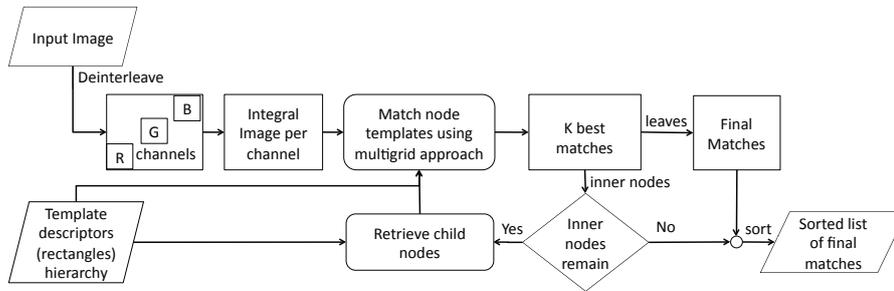
Figure 5.12: Workflow of our coarse-to-fine and hierarchical detection approach. First, the root node of the template tree is matched to the input image. Next, the  $k$  best match candidates are collected and further processed by matching the child nodes. Then, the  $k$  best candidates are collected again and the tree further traversed successively until the leaf nodes are reached. Leaf nodes represent a template each and lead us to the final matches.
