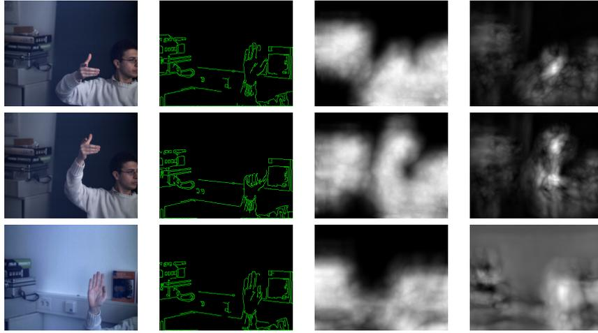
Figure 4.42: Test data set 3 is an open-closing sequence of the hand. Canny thresholds are 20 and 60
