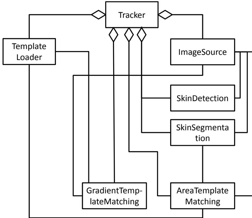
Figure 6.3: Class diagram of our most important classes of our hand tracking framework.
