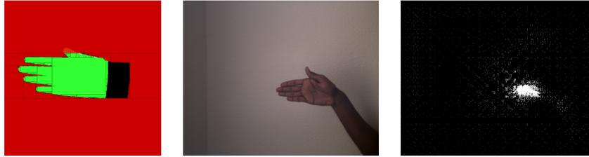
Figure 5.15: We match a template (left) to an input image (middle) using our multigrid approach. The confidence map (right) illustrates the actually evaluated positions in the input image. We can see that only a few positions have to be matches, which saves a lot of computation time.
