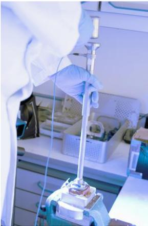
**Figure 8.20: Biomedical experimental setup.** A donor acetabulum is mounted to a vise, the real implantation tool is hammered into it, while data is recorded.
