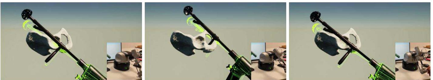
Figure 6.7: Arbitrary contacts. Any other configuration of the tool on the surface of the pelvis is possible. Even very unusual contact configurations (*Center*) can be stably rendered, without noticeable artifacts. Green shows the haptic tool (see [Section 6.3](#)).
