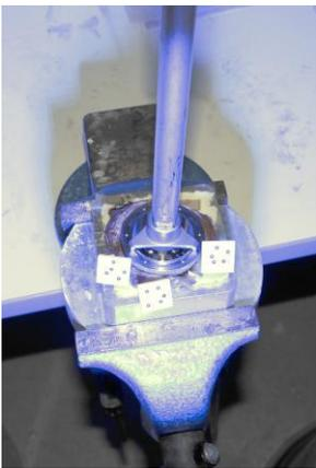
**Figure 8.21: Biomedical marker setup.** The organ pose is tracked by three markers, and the implant by another marker.
