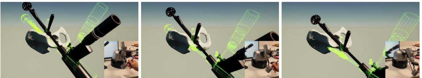
Figure 6.6: Smooth sliding. The other side of the shaft has no such features, and allows for smooth low-friction sliding along the top half of the pelvic bone. Green shows the haptic tool (see [Section 6.3](#)).
