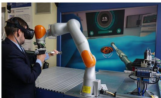
**Figure 9.** The Virtual Reality acetabulum reaming simulator, where the developed real-time material model is used to simulate the interactional forces and torques between the reamer and the acetabulum.
