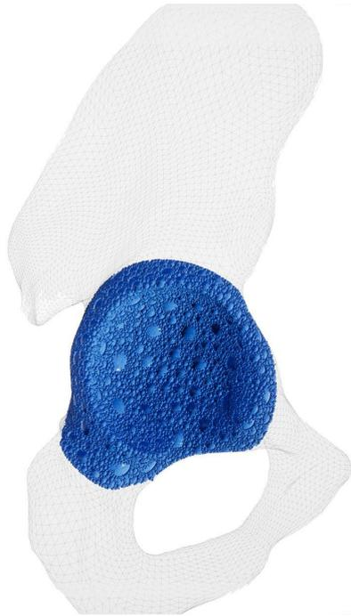
**Figure 8.** Example of a volumetric model of the acetabulum filled with spheres, which is used to calculate the force feedback given by the Virtual Reality simulator. The usage of spheres allows a fast computation of the force feedback.
