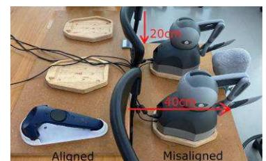
**Figure 9.1: Registration error.** The dimensions of the registration error: the real devices are translated towards the user by 40 cm and downwards by 20 cm. This introduces an inverse registration error, effectively moving the virtual tools away and upwards from the user, in resemblance of desktop-based virtual simulators.
