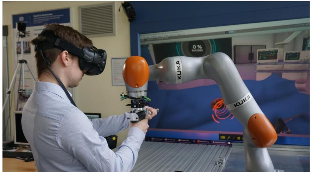
Figure 8.16: HIPS on Haption Virtuose. Showing someone using the HIPS simulator, on a Haption Virtuose.
