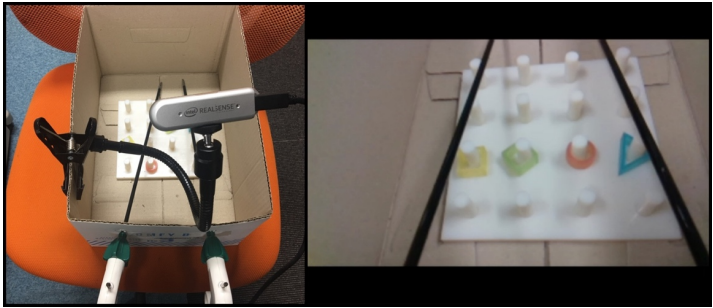
Figure 1: Left: setup of the box trainer. Right: camera view.
