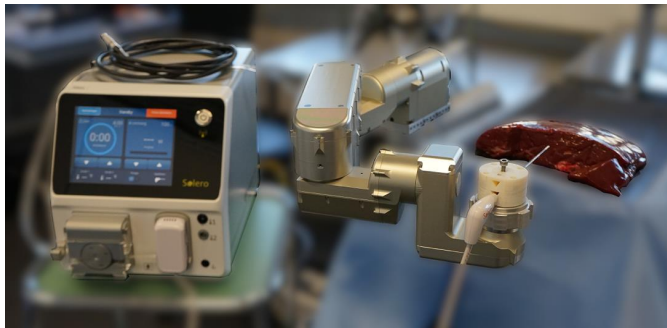
Figure 2: Experimental setup with the robotic device, the ablation system and ex-vivo bovine liver
