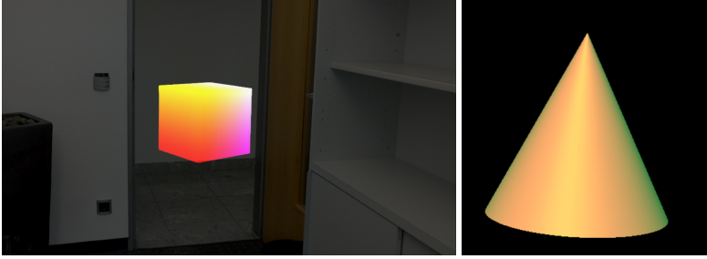
Figure 1: The content that was used for testing the different streaming approaches. The left image shows the view inside the HoloLens from the user's point of view. The cube was used for testing the 3DStreamingToolkit and HoloLens Remoting. The cone on the right side was used for testing JPG and DXT1. Both objects were animated during the streaming.
