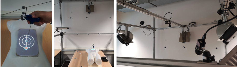
Figure 3: Experimental apparatus. Three projectors augmented a candle gel filled phantom with navigation visualisations. An IR-based optical tracking camera was used to obtain instrument position information.
