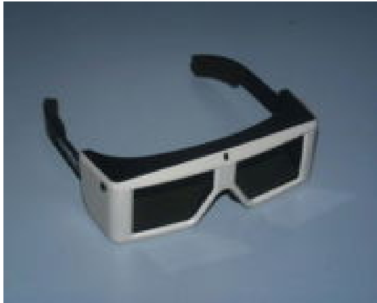
Figure 3.4: Active eye separation by shutter glasses
