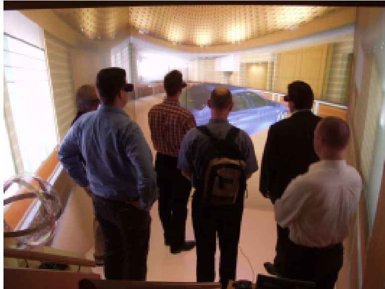
Figure 5.6: CAVE with 5 walls
