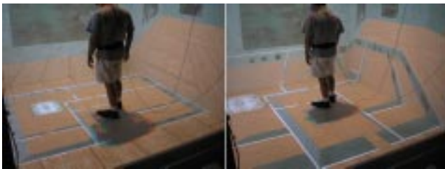
Figure 4 A user prepares to scale the Step WIM upward using the Interaction Slippers (left). As the user moves forward the Step WIM gets larger and his position in the miniature is maintained (right).
