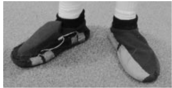
Figure 3 The Interaction Slippers allow users to tap either their toes or heels to trigger Step WIM functionality.
