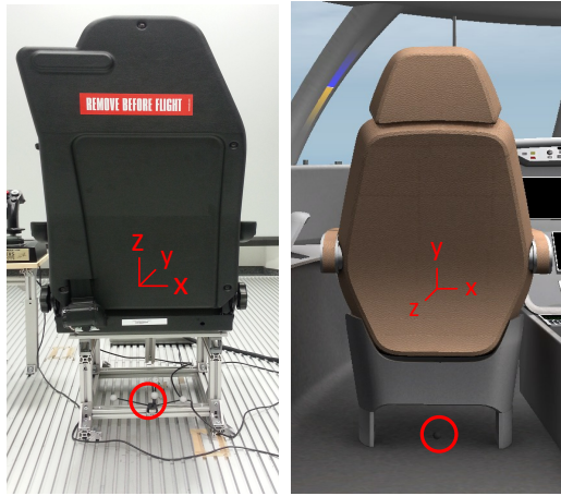
Figure 5: Alignment of the coordinate systems.
