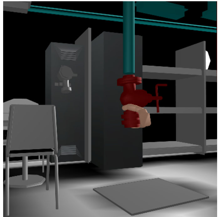
Figure 12. NEW PIPES CAN BE DESIGNED FROM BUILDING BLOCKS. HERE THE USER ATTACHES A VALVE TO THE END OF A NEW PIPE. WHEN THE VALVE TOUCHES THE PIPE AND IT HAS NEARLY THE “CORRECT” POSITION, THE SYSTEM SNAPS IT TO THE PIPE. DURING POSITIONING, COLLISIONS BETWEEN VALVE AND PIPE ARE HIGHLIGHTED BY RENDERING THE PIPE IN WIRE-FRAME. (DATA COURTESY .)
